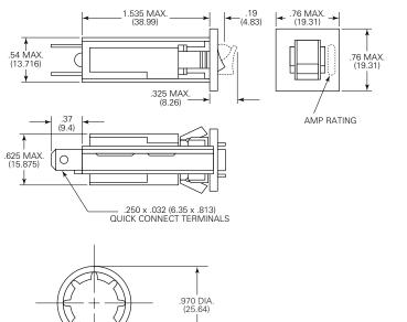
55-025B INTERNAL TOOTH PUSH-ON LOCKWASHER For panels greater than .105" (2.67) thickness
